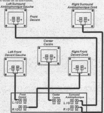
For normal operation of the VP ZERO, connect them to your amplifier's front channel output making sure that the positive (+) output form the amplifier is connected to the positive (+) input binding post on your speaker. Do the same with the negative (-) output and input. Use the supplied wrench to tighten the binding posts down on the wires and Bridging Bars.
